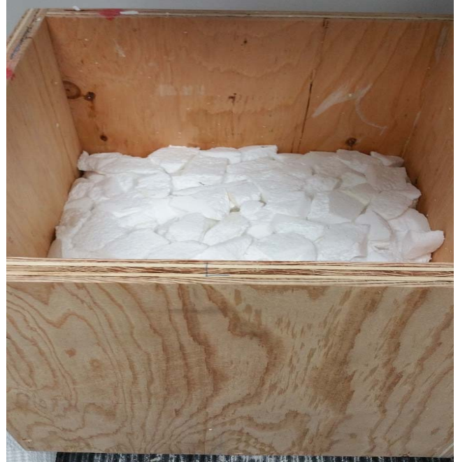
Figure 2 - EPS Loose Fill Material After Being Subjected To 9500 N Load
